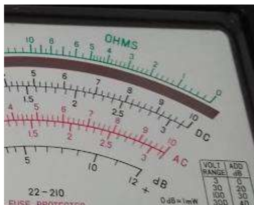
Analog multimeter showing different scale selections
