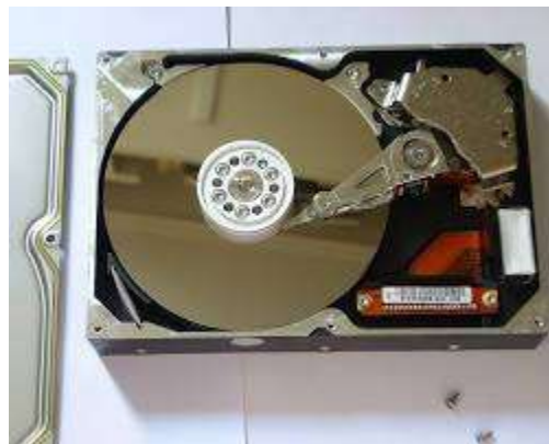
Hard drive showing magnetic platters
