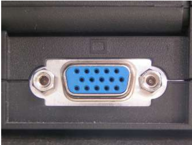
A picture of a VGA port.
