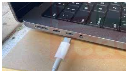
A picture of a USB Type-C port.
