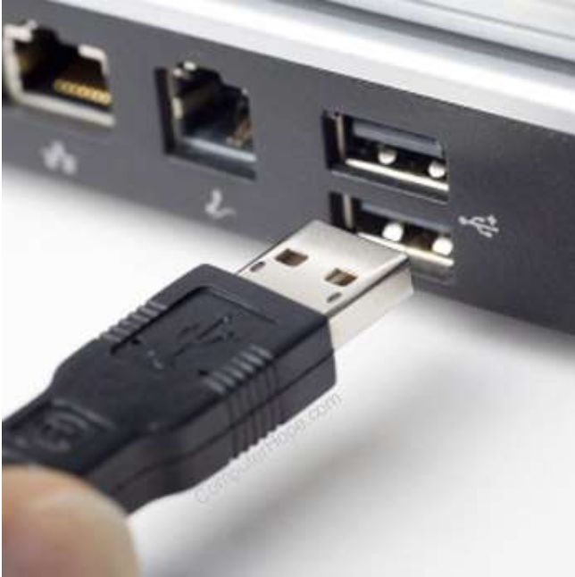
A picture of a USB Type-A port.
