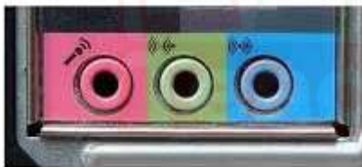
A picture of a 3.5mm audio output port (often green).
