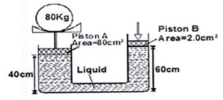
Determine the value of F needed to just lift the 80kg mass given the density of the liquid is 1.2g/cm<sup>3</sup>. (3 marks)
