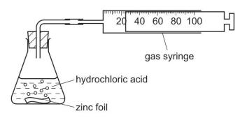
A piece of zinc foil was added to 50 cm<sup>3</sup> of hydrochloric acid, of concentration 2.0 mol/dm<sup>3</sup>. The acid was in excess. The hydrogen evolved was collected in the gas syringe and its volume measured every minute.
