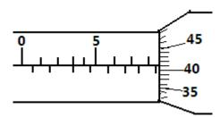
$M.S.R = 8.5 mm \checkmark$ S.S.R = (0.01 × 46) = 0.46mm \sim = 8.96mm \sim = 8. Actual reading = 8.96 - 0.5 = 8.46mm  $\checkmark$
