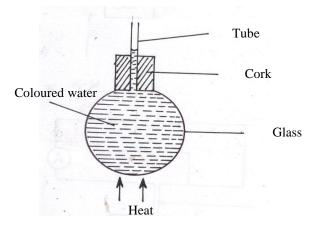
Glass flask expands first, creating more volume for water  $\checkmark$ . Water then expands increasing its level in the tube  $\checkmark$
