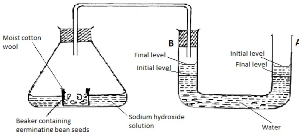
(a) After 48 hours the level of water in U-tube **A** had dropped and rose in **B** as indicated above. Explain this observation. (3mks)
