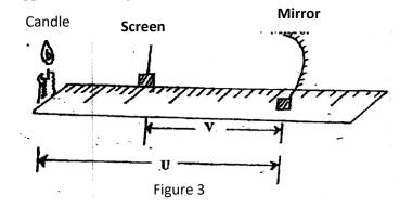
(g) Put th object at a distance u = 30cm from the mirror. Adjust the position of the screen until a sharp image is formed on the screen. Record the distance V.
