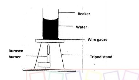
Measure 100cm<sup>3</sup> of water and pour it into the beaker. Take the initial temperature of the water.
