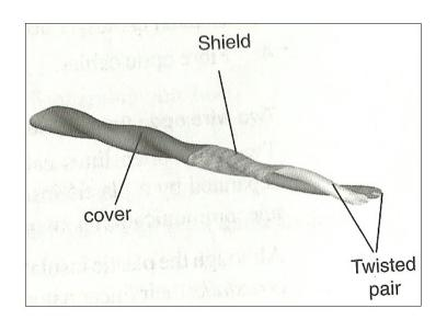
They have a braid wrapped around the wires to shield or protect them from noise.
