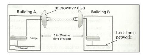
In microwave transmission signals travel in a straighteline and therefore the transmitter and receiver must be in a direct line of sight of each other.
