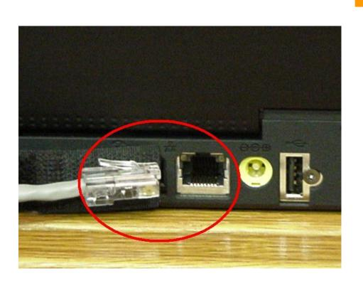
In this practical exercise, we are going to use twisted pair cabling technique because it has become almost the default method. This type of media uses a connector known as RJ45 to terminate the cable. Figure right shows illustration of RJ45 port and RJ45 terminated cable. RJ45t is attached to a UTP cable using crimping tool.
