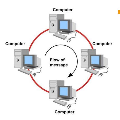
Ring topology – in this topology all the components are connected to a single cable forming a ring. The data flows in only one direction and the signal is actively retransmitted by each node to its neighbour if its not addressed to it.
