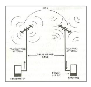
Radio waves travel just like surface water waves, i.e. they are *omnidirectional*. This means that they start from a central point and spread outwards in all directions. As they travel outwards, their energy spreads outwards over the covered area. The waves are radiated into the atmosphere by a radio frequency antenna at constant velocity. Radio waves are not visible to the human eye. Figure right shows a typical radio waves link between two separate geographical locations
