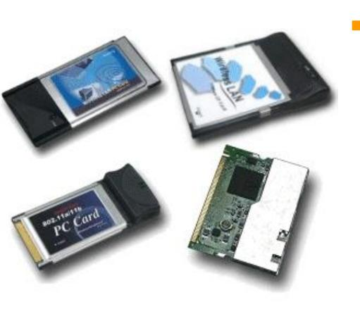
Personal Computer **Memory Card** International Association Cards – the PCMCIA is an add on card inserted into a device such as personal digital assis ants or a laptop in order to enable wireless communication between the devices and a wired network server.
