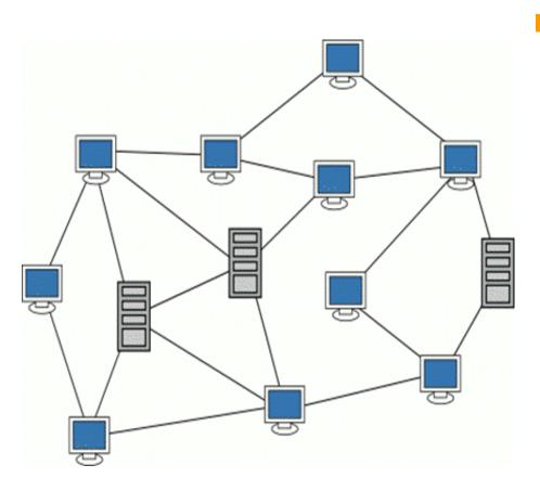
Mesh topology – this topology uses separate cables to connect each device to every other devices on the network providing a straight communication path.
