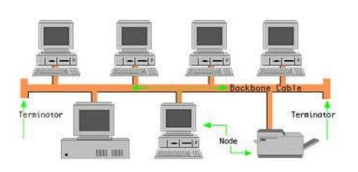
Bus topology – all devices are connected to a central cable called the bus or backbone. Transmission and reception of a message is done by all the hodes. However, only one node can carry out a transmission at any one time. 63
