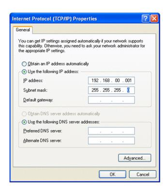
3. Type in the IP address such as 192.168.00.001. Each computer should have unique IP address. Figure right shows a TCP/IP properties dialog box in Microsoft Windows XP.
