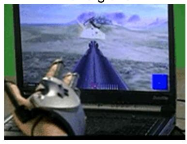
They are worn on the hands to allow the user navigate through the virtual world and interact with virtual objects. The gloves have sensors that collect data about the movement of the hands and relay the data into the system. They give the wearer a sense of touch in the virtual world.
