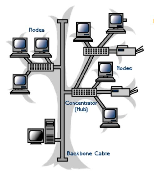
Tree/Hierarchical topology – all the nodes are connected in form of a tree with nodes as leaves and links as branches. The transmission medium is a branching cable with no closed loops. The branches in turn can have more sub-branches. Branches are connected to each other by means of devices called hubs.
