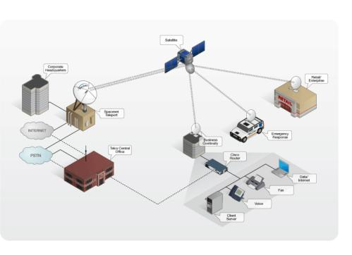
The new trends in microwave transmission have seen the use of very small aperture terminal (VSAT) technology. This refers to a very small satellite dish used both in data, radio and TV communication. Many businesses are adopting this new technology because it enables direct access to satellite communication instead of having to go the ough the state owned satellite gateway. Figure right shows VSAT technology as set up to enable two laptops in geographically disparate locations to communicate.
