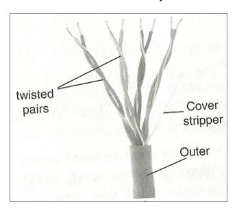
They do not have a shield the prevents electromagnetic interference hence they are susceptible to noise and signal interference.
