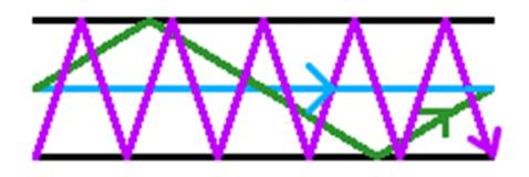
Multimode fibre – it has a thicker core and allows several light rays to be fed in the cable have a high attenuation rate and they are mainly used for shorter distance transmission. The light is bent back into the core hence propagates along the length of the cable as shown in figure right below.
