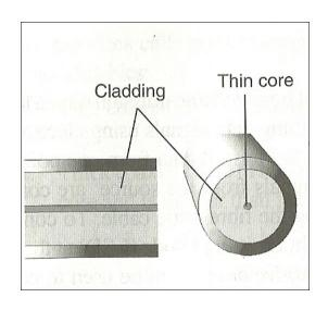
Single mode fibre has a very narrow centre core. The light in the cable therefore take only one path through it making to have a low attenuation rate.
