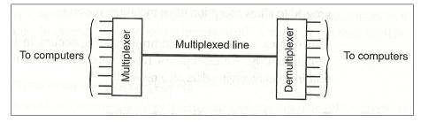
Multiplexing – it's a process of sending multiple data signal over the same medium while demultiplexing is the process of separating the multiplexed signals at the receiving end.
