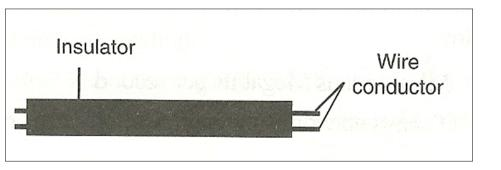
Are made up of two parallel copper wires separated by a plastic insulator as shown figure right. They are used in telecommunication network to transmit voice signal.
