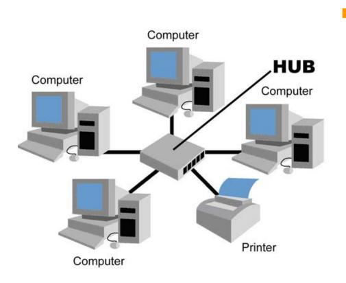
Star topology – in this topology, all devices are connected to a central hub. Workstations communicates across the network by passing data through the hub. When the hub receives data from a transmitting computer, it broadcasts the message to all the other workstations on the 55 network.
