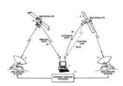
Intercontinental transfer of data is achieved by having satellite base stations transmitting the data through a wireless uplink channel to the satellite. The satellite then sends the data signal to the base station on another continent where it is picked up and sent to telephone exchanges for transfer to the destination computer. Figure left shows a logical local and intercontinental connectivity.
