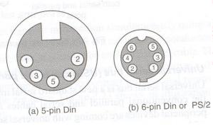
connector as the new standard to connect PS/2 mouse and keyboard. Figure 2.26 shows a 5-pin and PS/2 connectors showing physical difference in size. I
