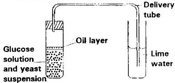
Glucose solution was boiled and oil added on top of it. The glucose solution was then allowed to cool before adding the yeast suspension.
