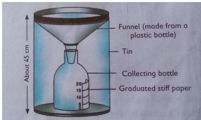
It is dug 15cm below the ground to prevent evaporation and to provide firm support.
