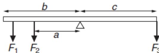
When the beam is released, the right-hand side of the beam starts to go down. Which of the three distances,  $a$ ,  $b$  or  $c$ , should be decreased in order to balance the beam? Explain your answer.
