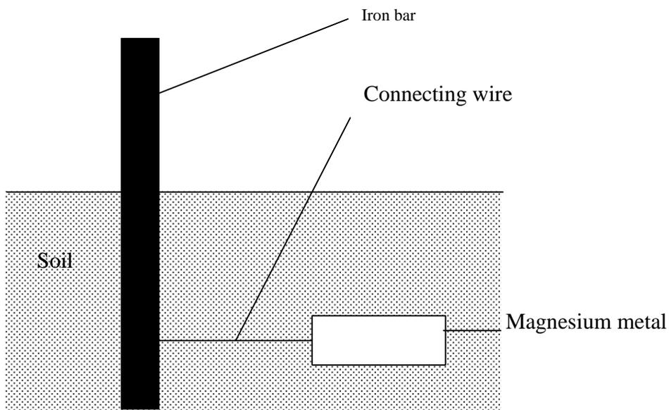
Explain why it is necessary to connect the piece of magnesium metal to the iron bar. (3mks)
