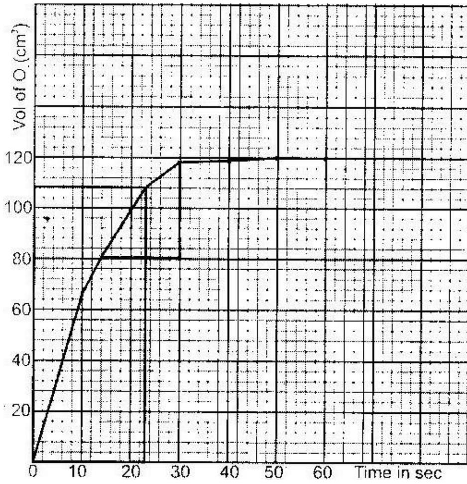
$$\text{iii) Rate of O}_2 \text{ production} = \frac{14\text{cm}^3}{10\text{sec}} = 1.4\text{cm}^3/\text{sec}$$
