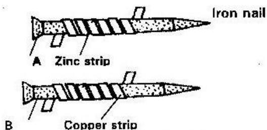
What observations would be made at the exposed points A and B if the wrapped nails are left in the open for several months? Explain. (3mks)
