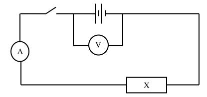
b) Record the voltmeter reading E when the switch is open.
