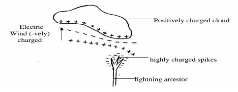
The arrestor acts as an easy way of discharging the clouds because it is a good conductor; ✓
