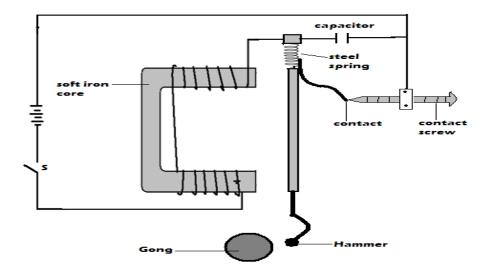
When circuit is closed, soft iron core gets magnetized and attracts the soft iron ammarture. The hammer being attached to the armature thus strikes the gong. the contacts breaks, core looses magnetism and armature returns to normal position. The process repeats.
