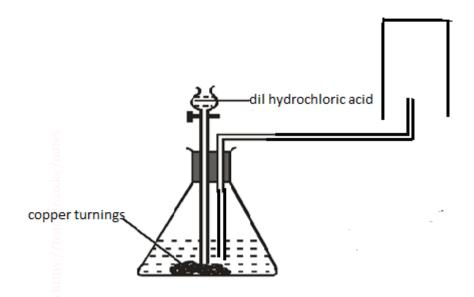
i) Identify two mistakes in the set up above.
