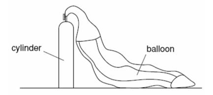
The balloon contains no gas initially. When it is connected to the cylinder, gas enters the balloon. The pressure in the cylinder decreases.
