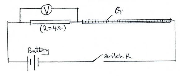
i. Use the voltmeter provided to measure the p.d  $V_R$  across R and the p.d,  $V_G$  across G when the switch is closed.
