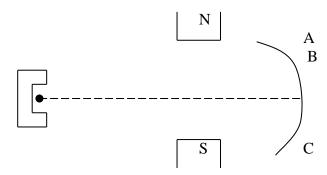
The background radiation at the place is 5 counts per minute. The detectors are placed a positions A, B and C respectively. Results obtained are shown in the table below.
