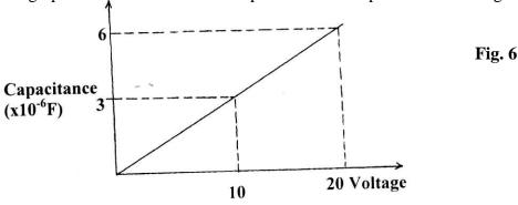
Use the graph to determine the quantity of charge stored in the capacitor. (3marks)
