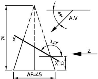
14. Make an isometric drawing from the three views given in Fig 10 below taking point X as the lowest point. (15 Mark)
