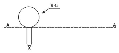
If the cup is rolled on the surface AA for one complete revolution, construction the locus of point X on the handle. (15 marks)
